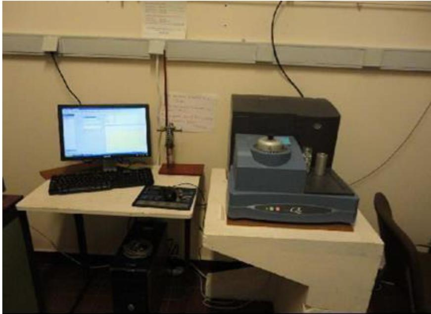
**Figure (II.4) :** DSC Q20 (TA Instruments).[2]
