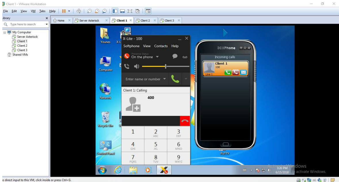
Figure.IV.20:Successful test call among extensions.
