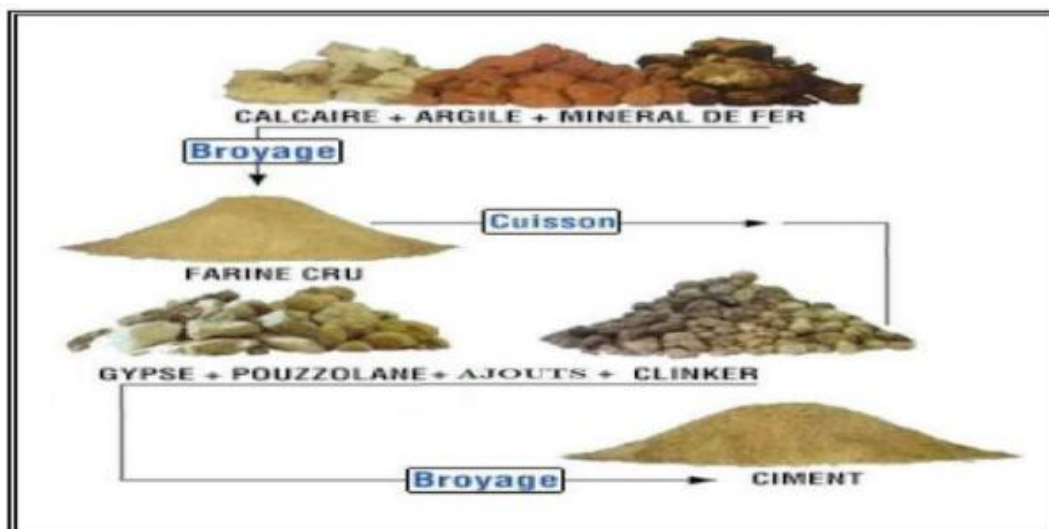
Figure I.1 : Cycle de fabrication ciment.
