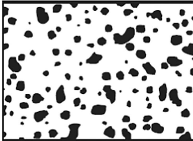
Figure 1.19 Two-phase material with particulate microstructure [15].
