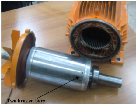
Fig. 2. The rotor with two broken bars.
