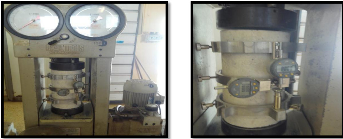
Figure.2.21. Experimental set-up of stress-strain measured during compressive test.
