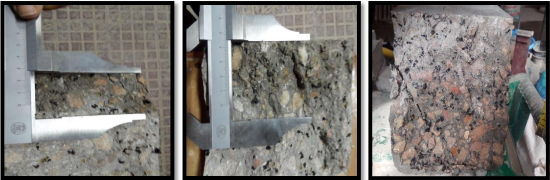
Figure 2.54. Depth of penetration of pressurized water of GC-based concretes of 10RW, 20RW and 40RW respectively.
