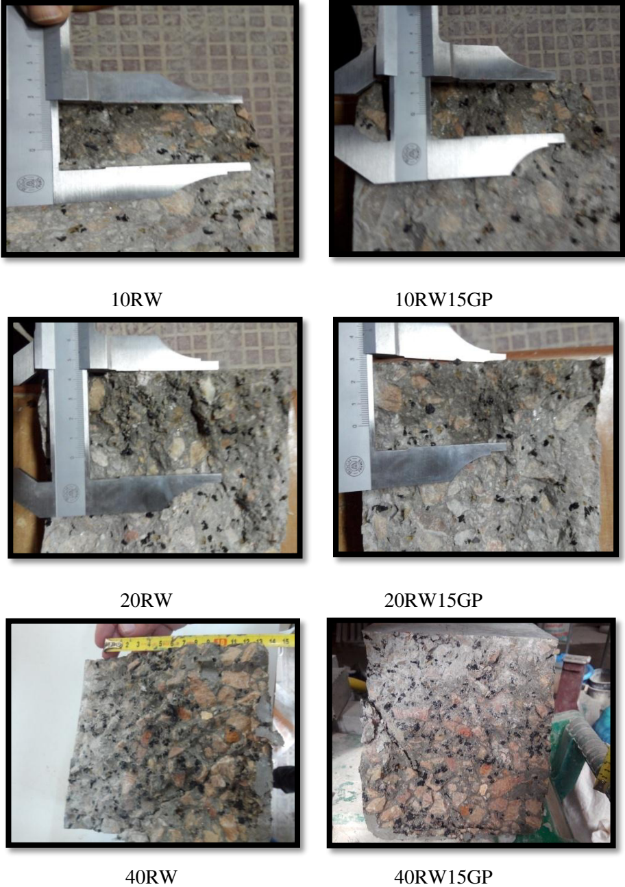
Figure.3.17. Depth of penetration of pressurized water of RW+GP-based concretes of 10RW, 20RW and 40RW respectively.
