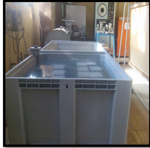
Figure.2.18. Water Curing of the mixtures.
