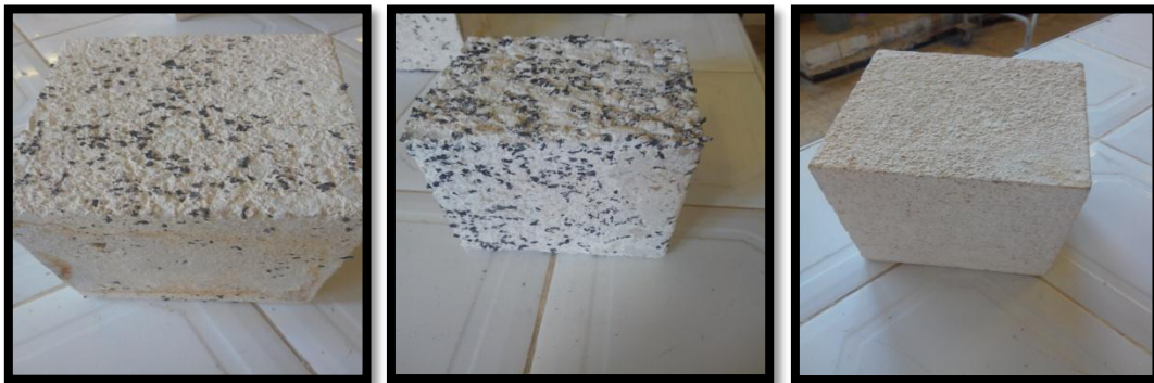
Figure.2.49. 28 days 40RW, 60RW, 0RW15GP acid attacked specimens respectively.
