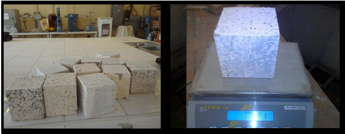
Figure.2.22. loss weight of specimens immersed in sulfuric acid.
