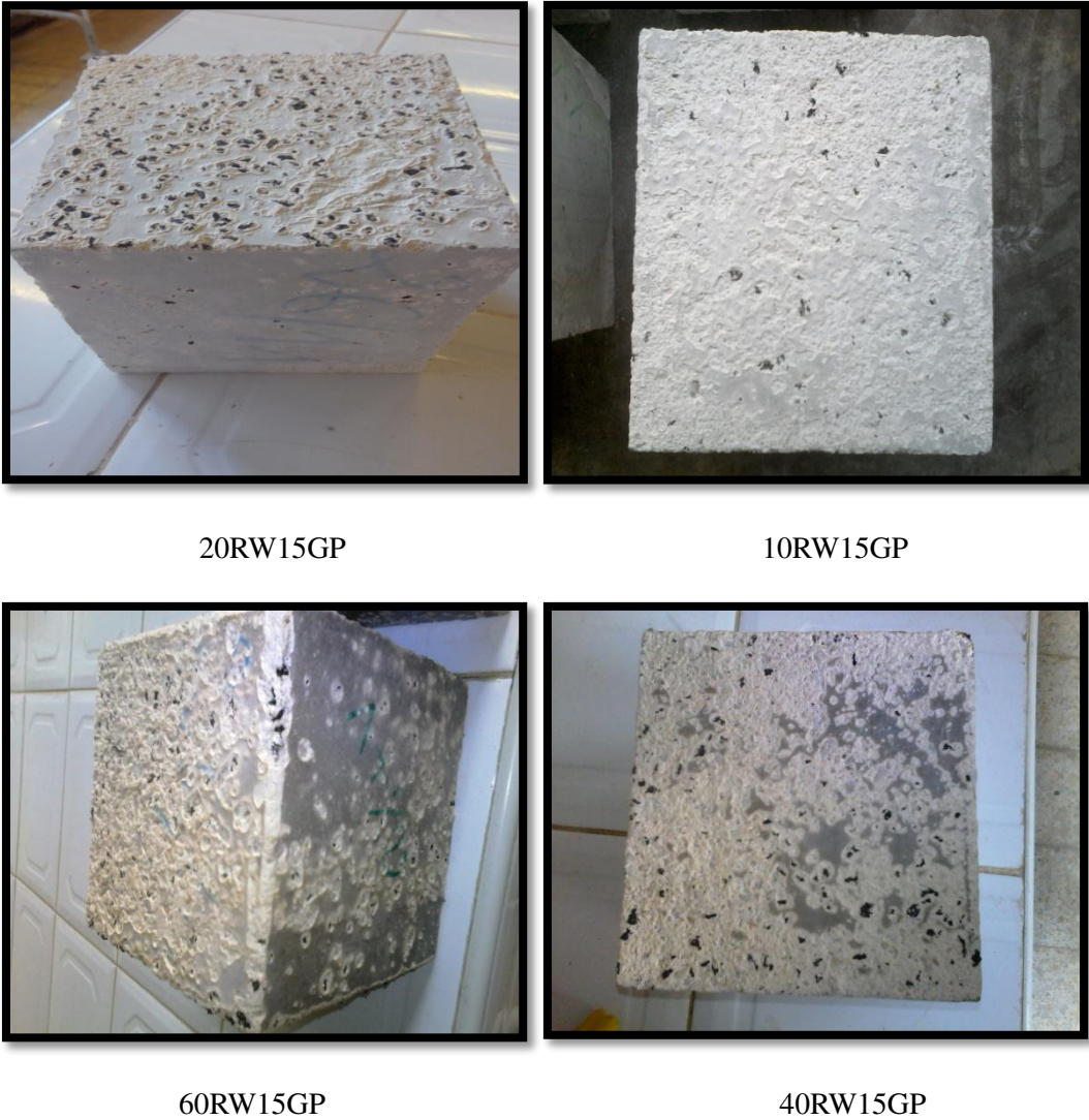
Figure.3.14. compined (RW+GP) wastes specimens immersed in sulfuric acid at 28 days.
