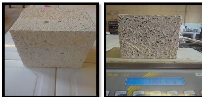
Figure.2.50. 28 days 0RW15SP acid attacked specimens and the aspect of measuring weight.
