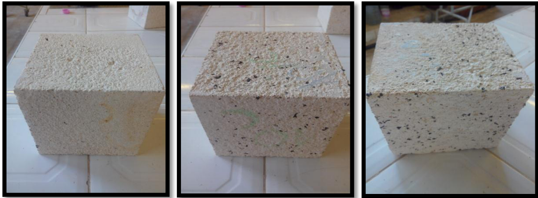
Figure.2.48. 28 days C-ref, 10RW, 20RW acid attacked specimens respectively.
