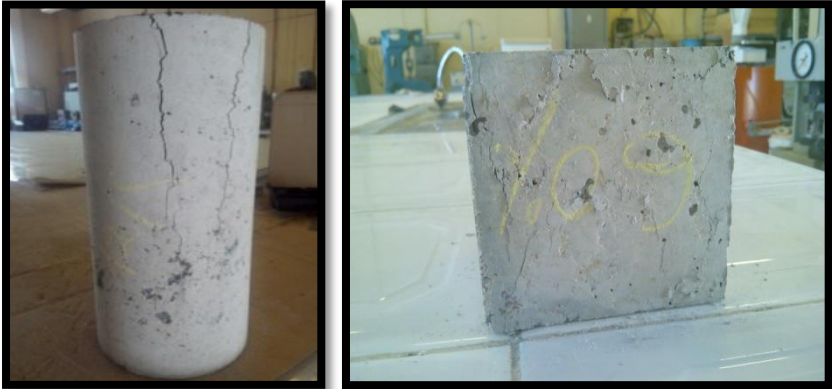
Figure.2.36. Failure pattern of 60RW concrete specimens.
