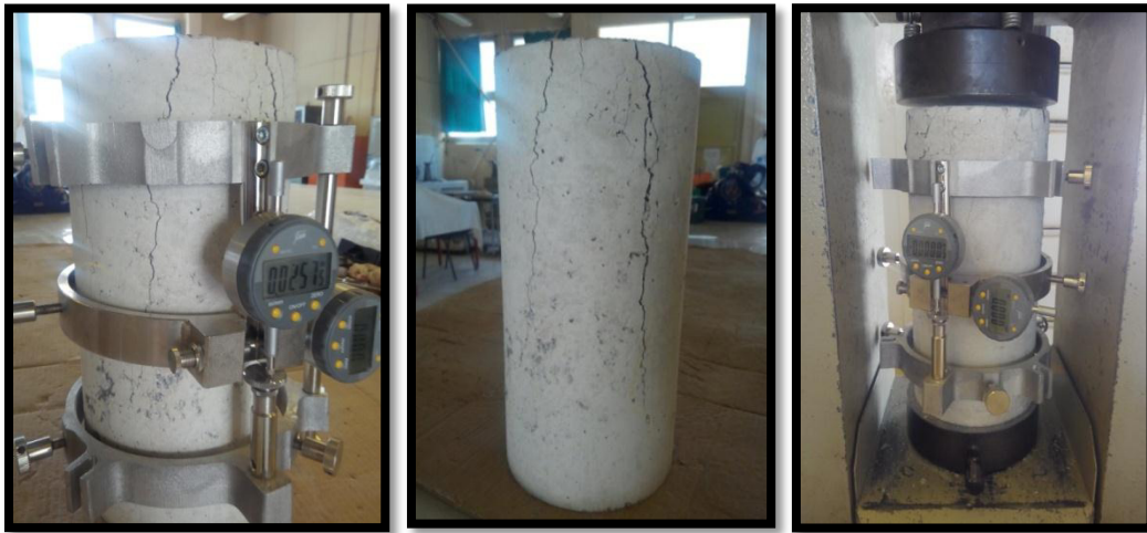
Figure.2.45. Physical appearance of rubber concrete specimens under the deformability test.
