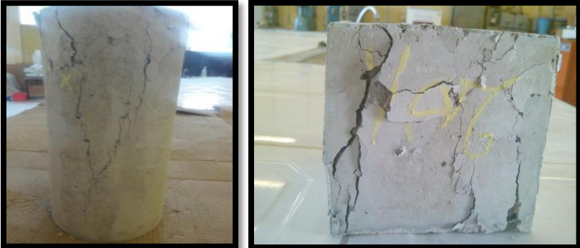
Figure.2.34. Failure pattern of 20RW concrete specimens.
