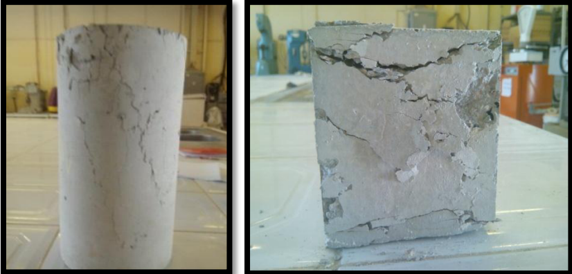
Figure.2.33. Failure pattern of 10RW concrete specimens.
