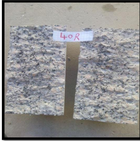
Figure.2.16. The dispersion of rubber aggregates in the composite.
