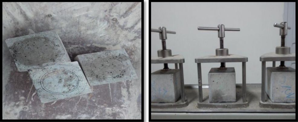
Figure.2.55. Experimental aspect and specimens of water permeability.
