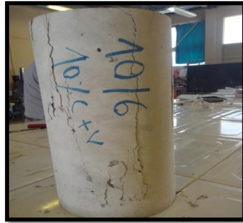
Figure.2.19. Machine used for compression test. Figure.2.20. Specimens after compression test.
