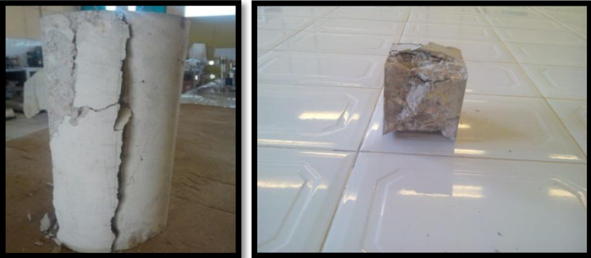
Figure.2.32. Failure pattern of reference concrete specimens.
