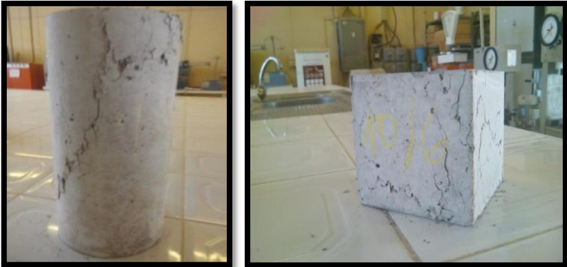
Figure.2.35. Failure pattern of 40RW concrete specimens.
