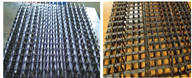
Figure 2.9: types de géogridles 3D.
