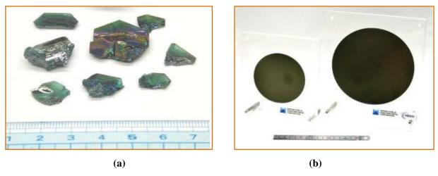
**Figure 1.1.** (a) SiC platelets (mainly 6H-SiC) obtained as a by-product in the Acheson process. (b) 4H-SiC wafers with 100 and 150mm in diameter [29].
