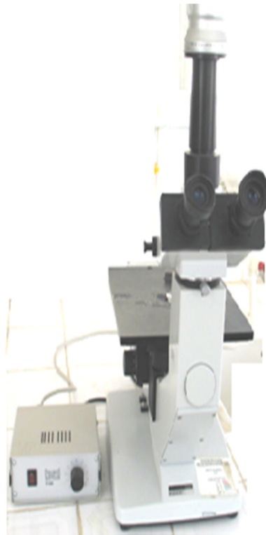
Figure II.3: Microscope optique de type Hund
