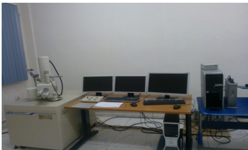
Figure. II.6: Microscope Electronique à Balayage de type JEOL-JSM-6390 LV
