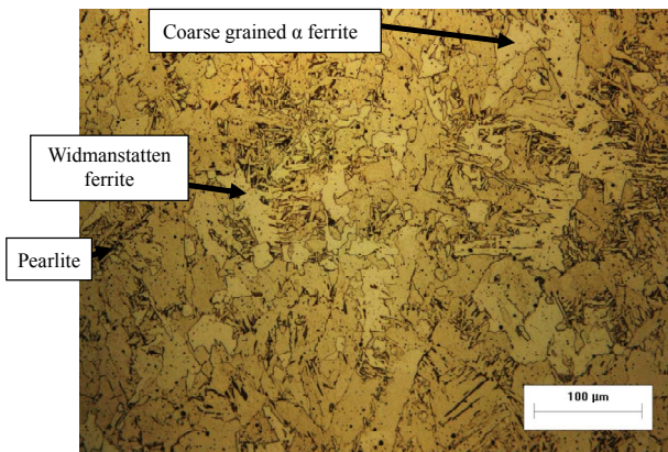
Figure 5. Microstructure of HAZ after welding of an industrial low carbon steel (0.19 wt. % C).
