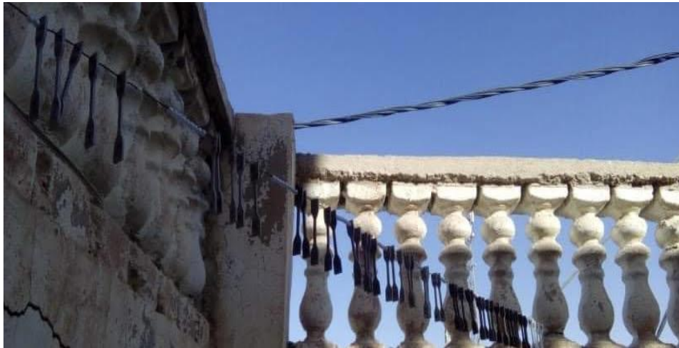
Figure I.12 : Experimental set-up for neat LLDPE, treated and untreated composites on natural weathering test
