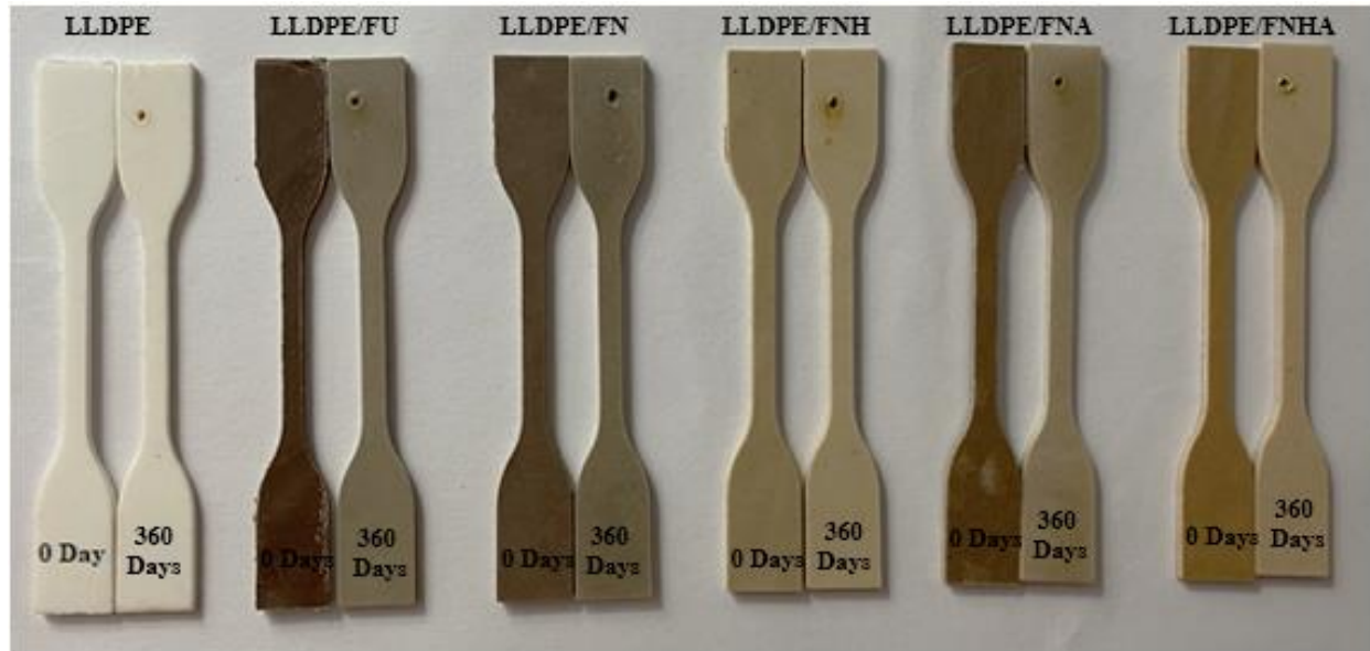
Figure III.1: Color change evolution of neat LLDPE, treated and untreated composite after 1 year of natural weathering
