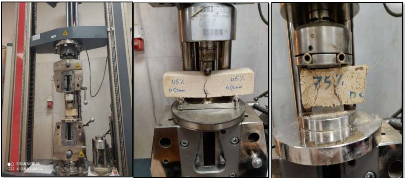
Figure 3. 7: Mechanical test device (bending and compression behavior)
