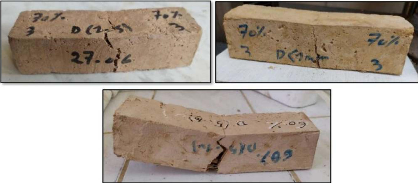
Figure 4. 41: Specimen after failure under flexural test.
