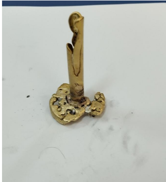
Figure III.6: A copper sample obtained by the continuous casting machine.
