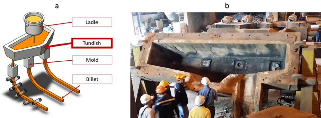
Figure II.4: (a)Diagram of continuous casting process(b)The 4-strand tundish at Millcon Steel PLC, Thailand [6].
