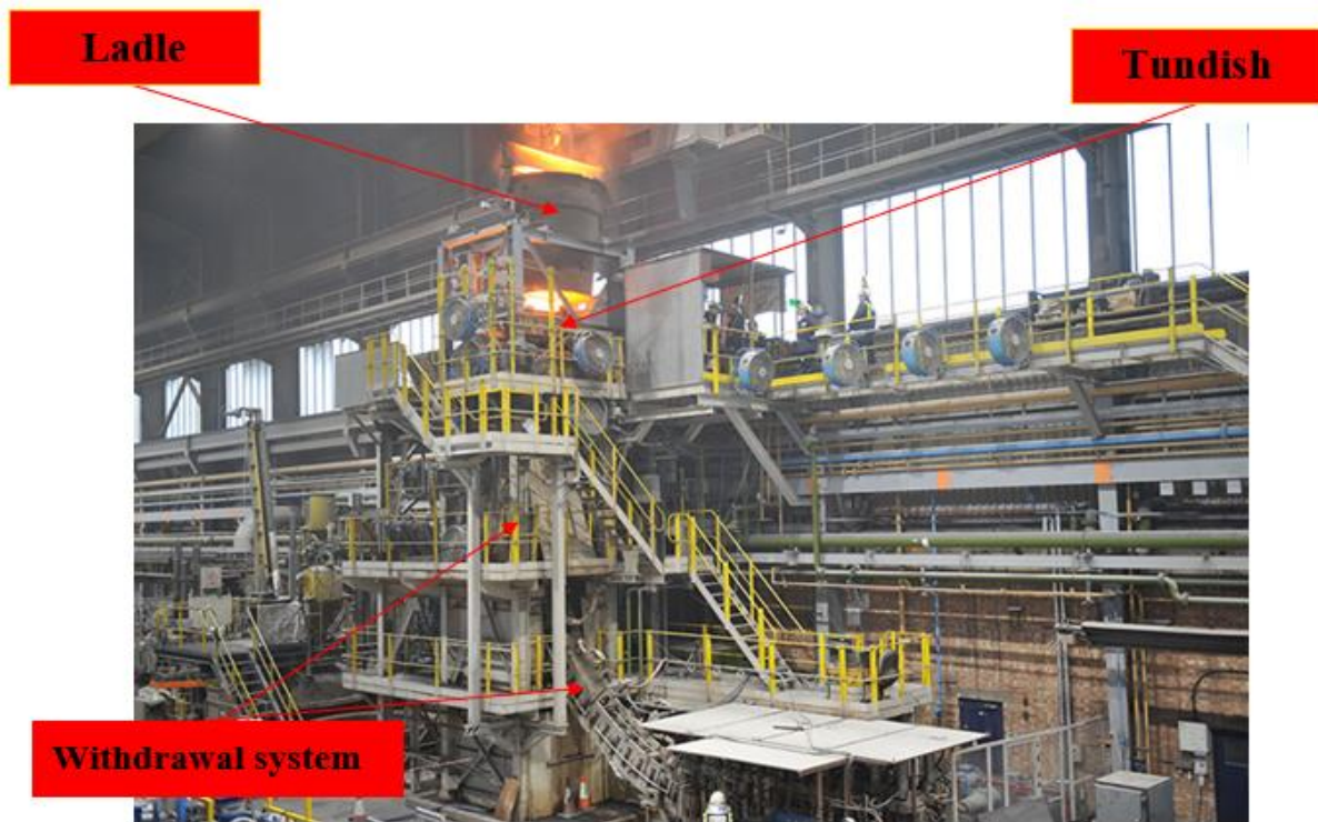
Figure II.2: Vertical downward continuous casting machine [3].
