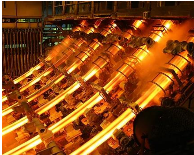
Figure II.7: The secondary cooling [10].
