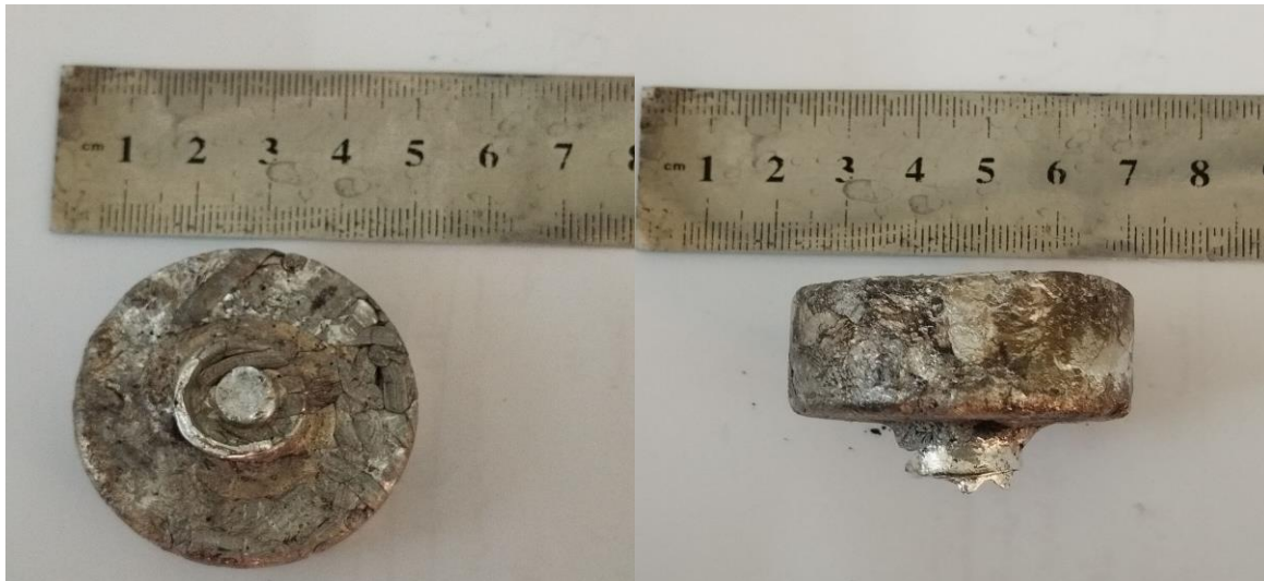
Figure III.7: Aluminum alloy sample manufactured by the continuous casting machine.
