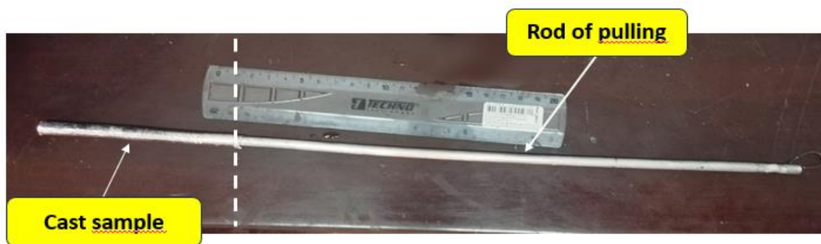
Figure III.14: Aluminum alloy cast sample manufactured by continuous casting machine under mechanical vibration.
