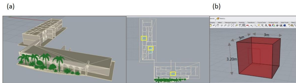
Figure 5.1: (a) Base case modelling design and situation of studied patient rooms in perspective and top views in Rhino; (b) patient room model parameters in Rhino (Source: Author, 2021)
