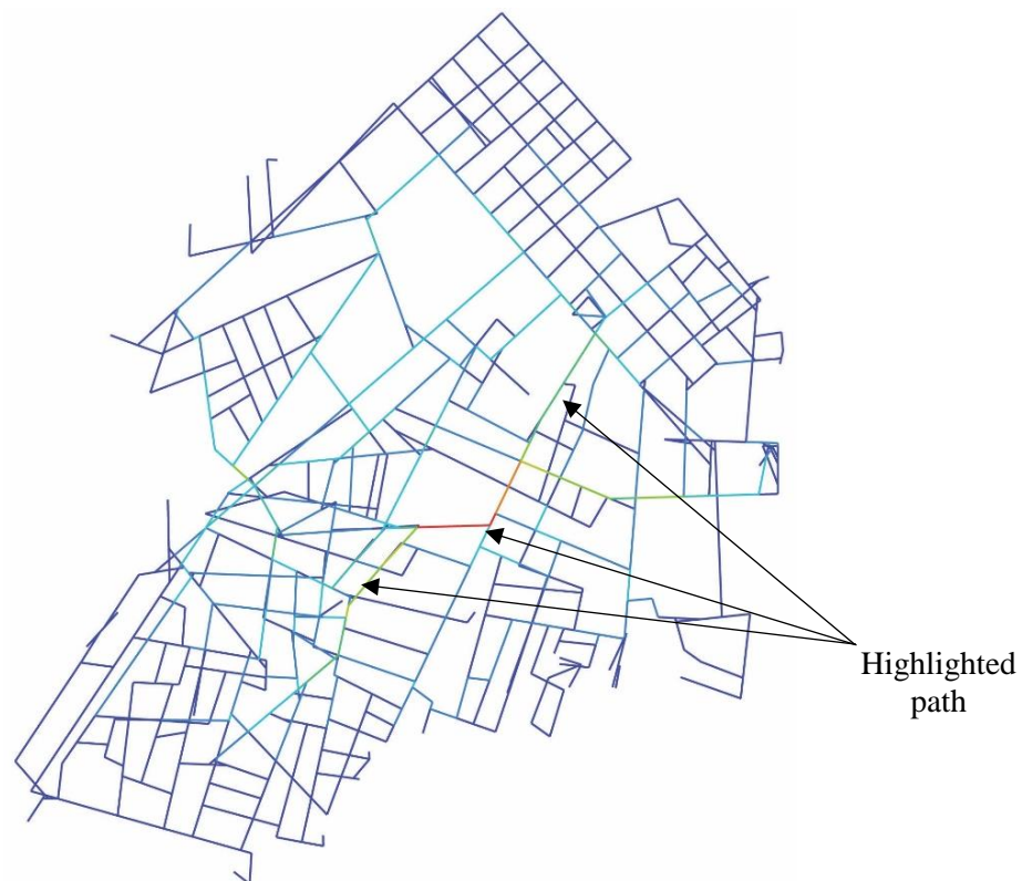
Figure VI.11. The metrical segment map of the city centre with the global radius R_n .
