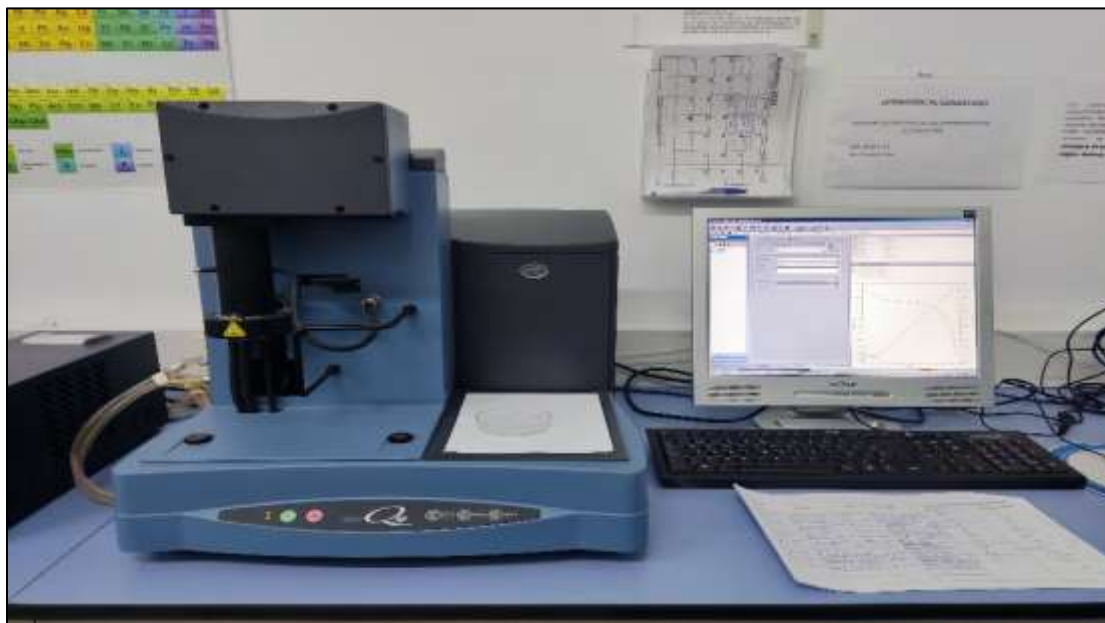
Fig. II.7. The used device for the thermal degradation analysis ( University of Cadix, Spain ).
