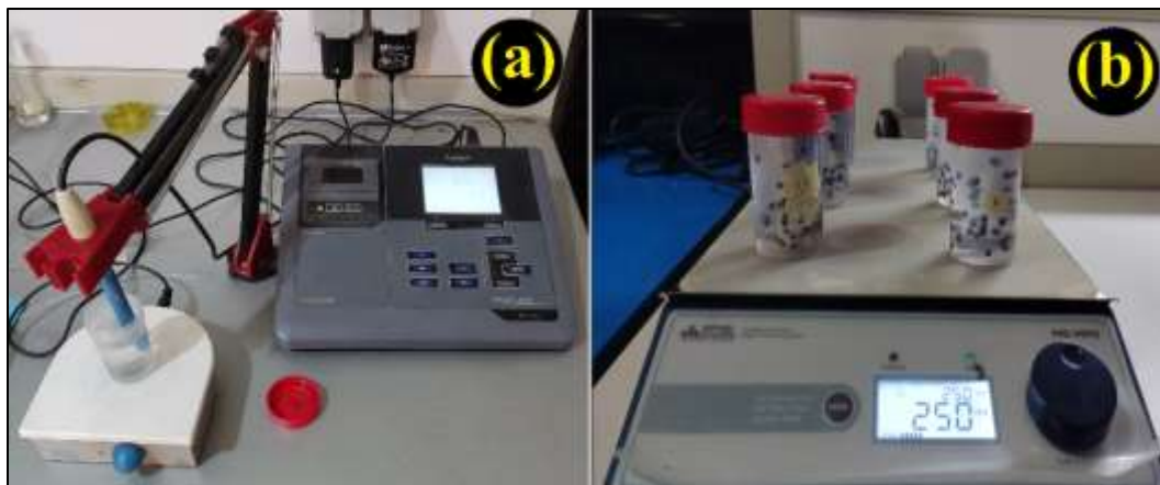
Fig. II.9. (a) pH meter device and (b) pH PZC experiment.
