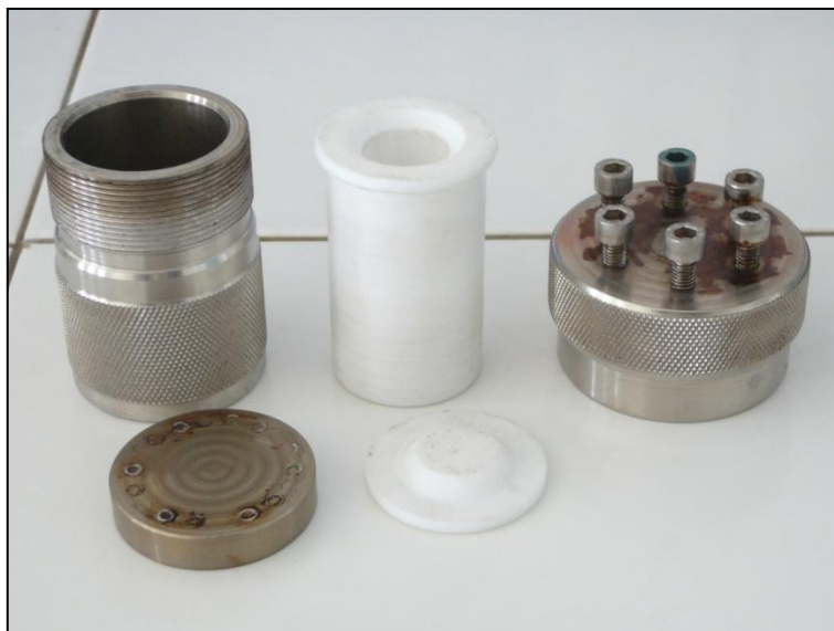
Figure II.2 : Autoclave de 23 ml de fabrication locale.
