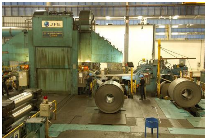
Figure 8 : Train de laminage
